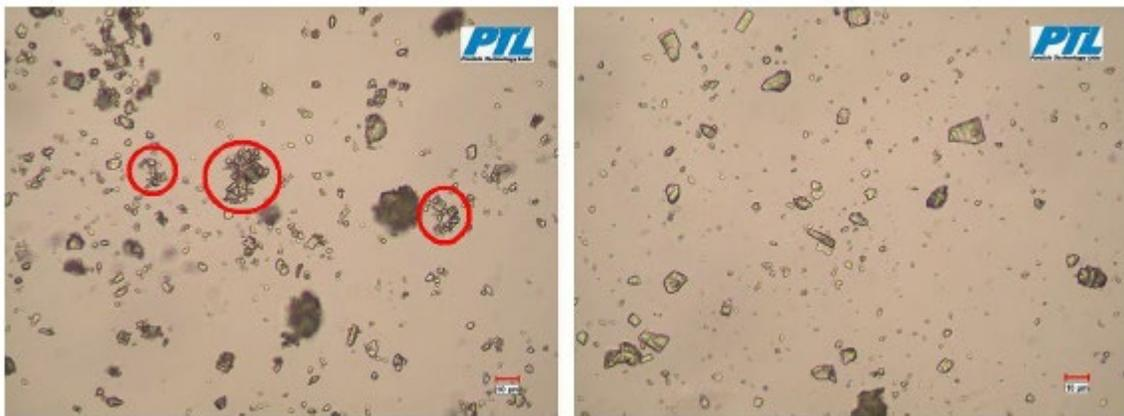
FIGURE 9. Flocs emphasized by the red rings in an unstable dispersion (left) which are not present in a stable dispersion (right)
