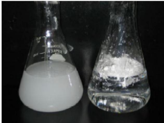
FIGURE 4. Dispersion of magnesium stearate into 2-propanol (left) and water (right).
