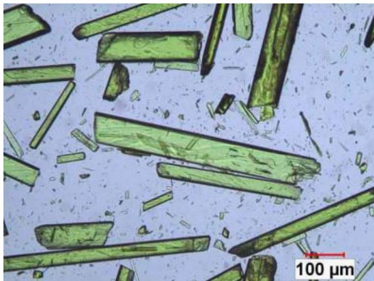
*Figure 2: Acicular particles are not recommended for laser diffraction analysis. Image analysis is a better option for particle characterization.*
