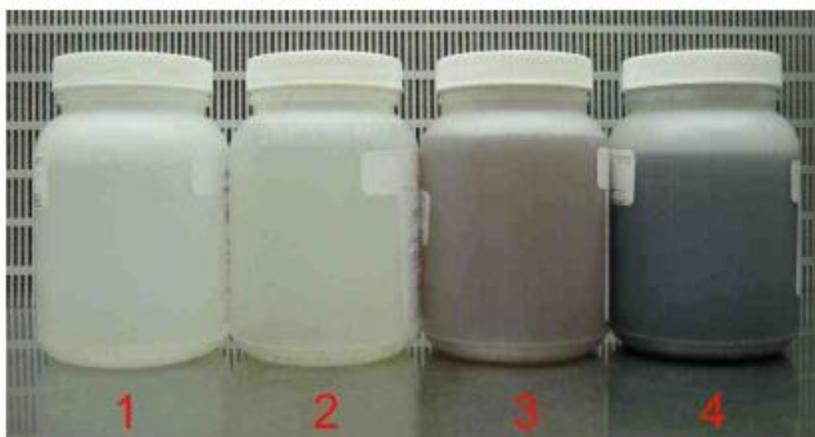
*Figure 8: Samples 1 and 2 required light obscuration analysis due to their dilute nature. Samples 3 and 4 were also analyzed using light obscuration in order to acquire results comparable to samples 1 and 2 on both a number and volume weighted basis.*
