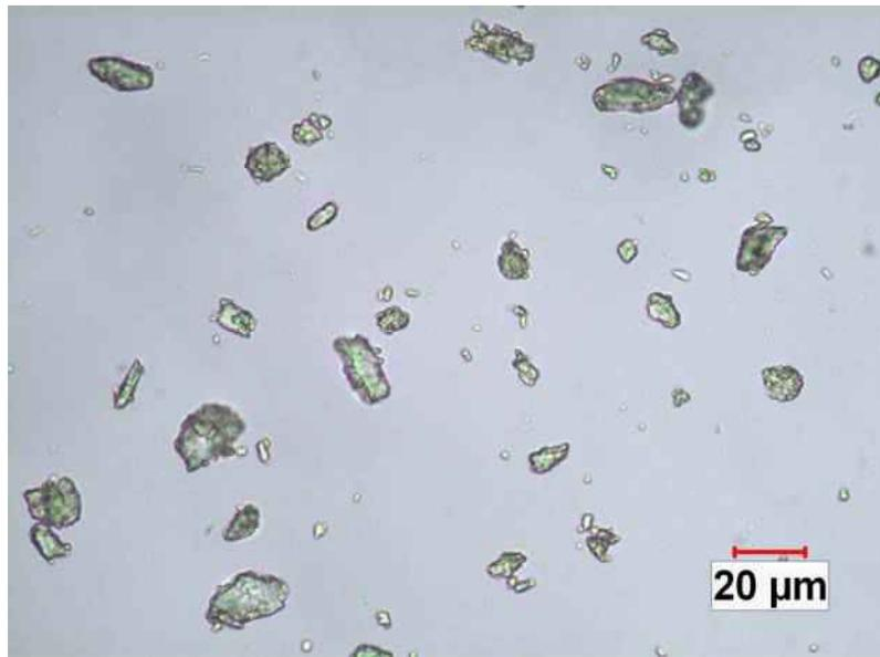
**FIGURE 14.** Photograph of particles from Figures 12 and 13. While submicron particulate is difficult to photograph due to the limits of optical microscopy, it can be observed as a haze or blinking on a live wet slide when viewed by microscopy. Nevertheless, it is unlikely that the distribution in Figure 12 is a realistic depiction of the particles in this sample.
