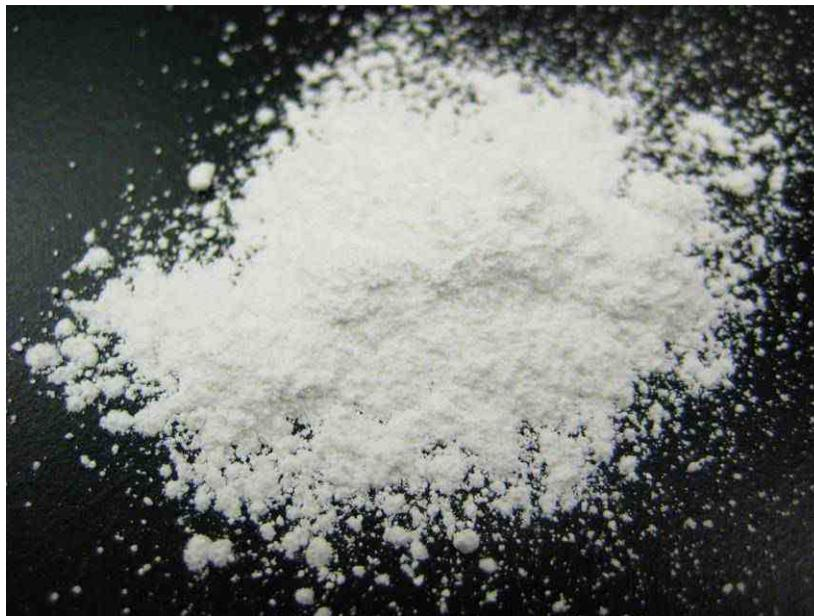
**Figure 1: This sample type benefited from sieve analysis due to the presence of soft agglomerates that indicated lot acceptability.**
